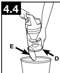
Close dirt cup door (E). Press firmly to secure.
