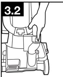
3.2 To remove hose for tool use, press the hose release button and pull hose end out.
