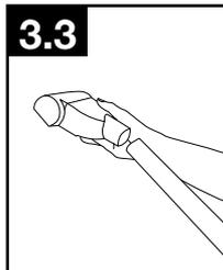
3.3 To attach tool or wand to hose, push firmly into place.
