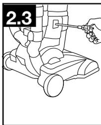
2.3 Prior to using, grasp the end of the plug and pull to release the cord from the cord reel until red tape is reached.
