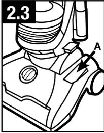
2.3 For optimal cleaning performance on bare floors and carpet with pile deeper than 1", brushroll should be turned off.
