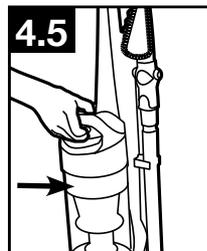
4.5 Place bottom of dirt cup into vacuum body first. Pivot dirt cup into vacuum body and press firmly until it locks into place.
