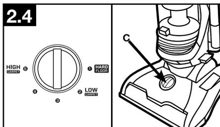
2.4 To adjust height setting, PUSH DOWN and TURN knob (C) to desired height setting.
